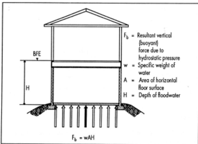
Figure 6. Buoyancy Force
