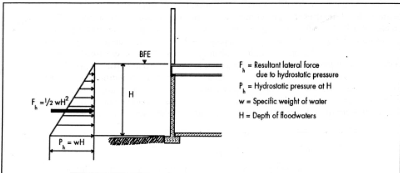
Figure 5. Lateral Hydrostatic Force and Pressure
