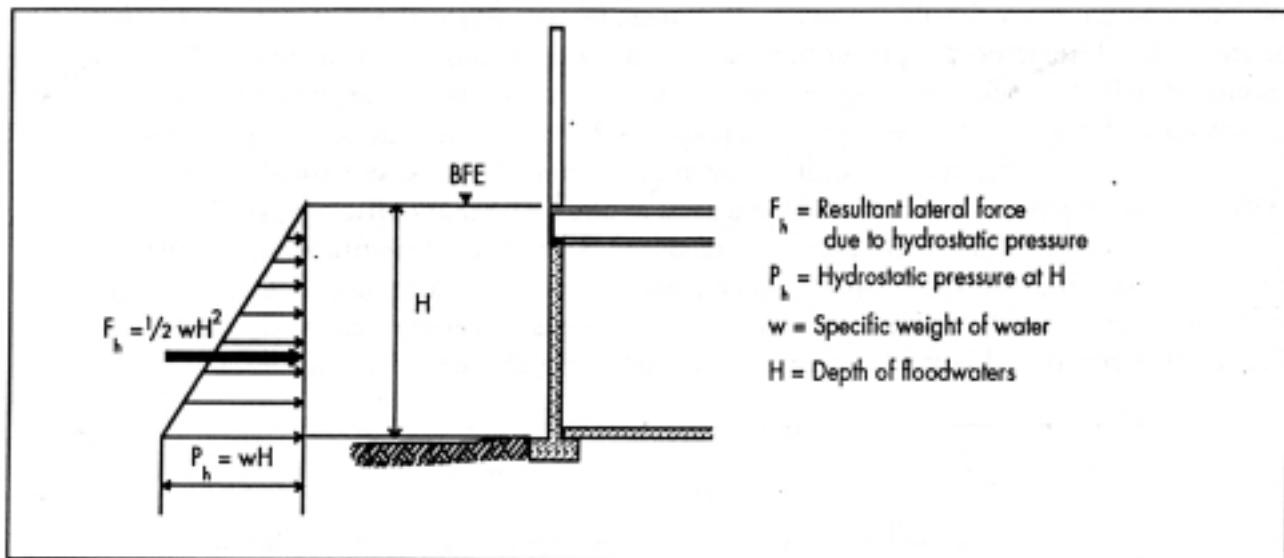
Figure 5. Lateral Hydrostatic Force and Pressure
