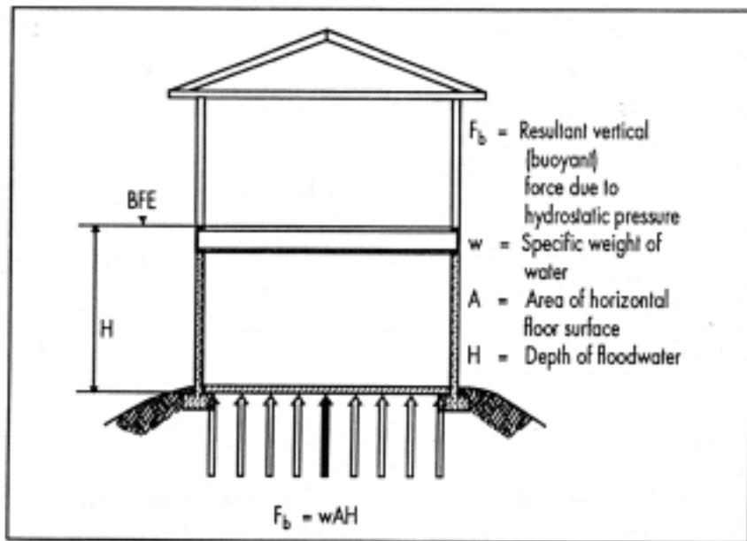
Figure 6. Buoyancy Force
