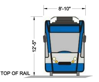
*Figure 2: Typical LRT Dimensions (overhead catenary wires not shown or included in the dimensions)*
