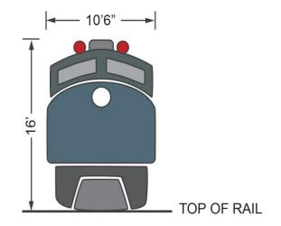
Figure 3: Typical CRT Dimensions
