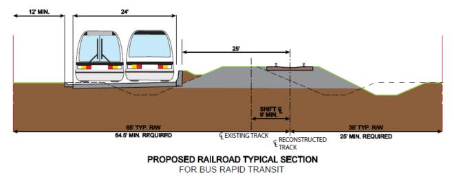
NOTE: ADDITIONAL R/W WOULD BE REQUIRED FOR STORMWATER TREATMENT PONDS
