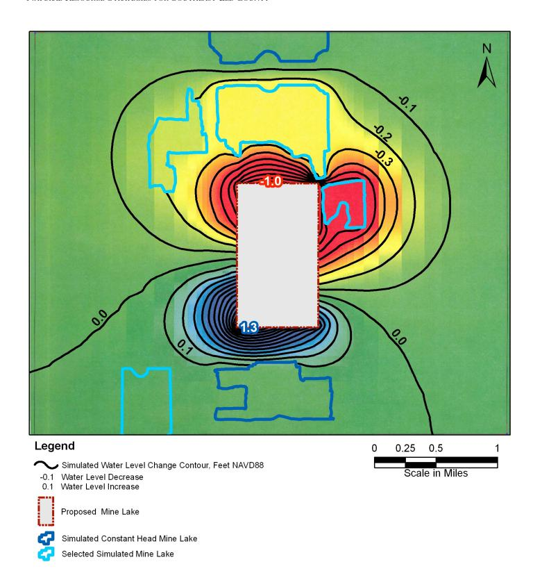
Figure 4.6: Simulated Contours of Water Level Changes for Scenario 1 4.12
