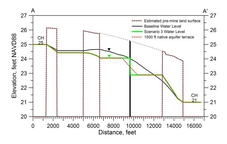
Figure 4.15: Profile of Groundwater Levels Comparing 1,500-foot-wide Native Aquifer Terrace versus Slurry Wall
