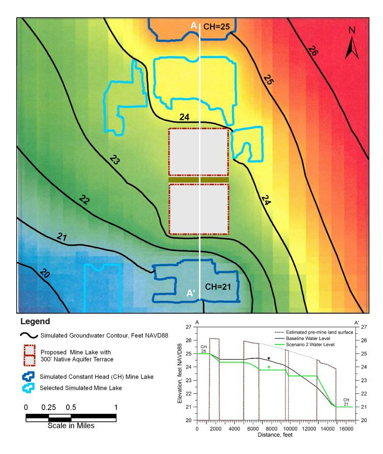
Figure 4.7: Simulated Contours and Water Level Profiles of Groundwater Elevation for Scenario 2
