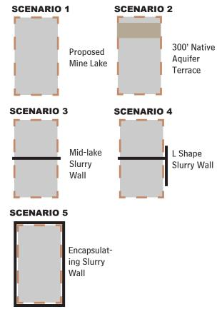
Figure 4.3: Schematic of Innovative Mining Concepts
