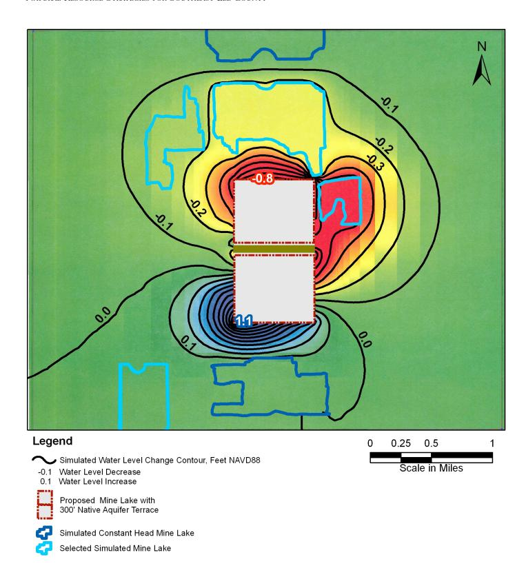
Figure 4.8: Simulated Contours of Water Level Changes for Scenario 2
