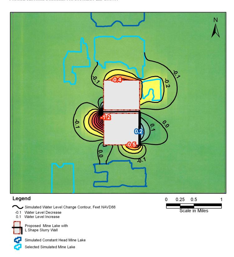
Figure 4.12: Simulated Contours of Water Level Changes for Scenario 4  $4.20\,$
