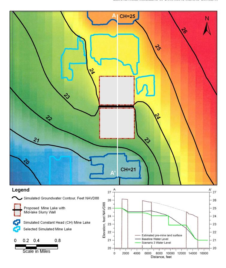
Figure 4.9: Simulated Contours and Water Level Profiles of Groundwater Elevation for Scenario 3
