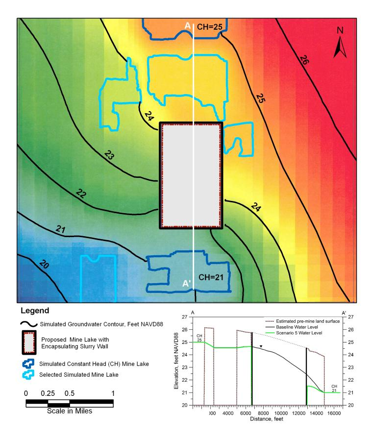
Figure 4.13: Simulated Contours and Water Level Profiles of Groundwater Elevation for Scenario 5
