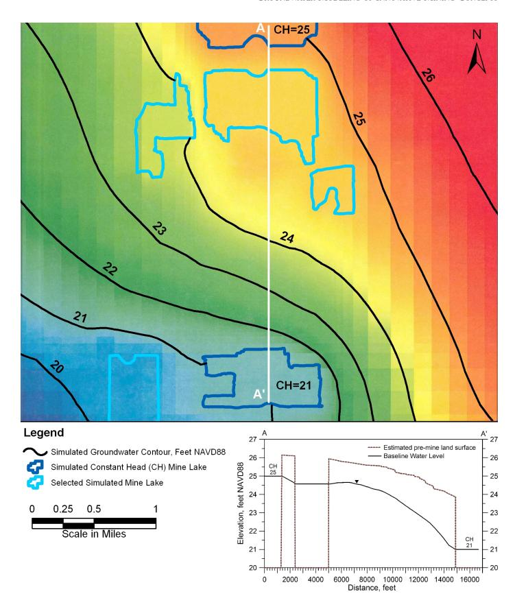
Figure 4.4: Simulated Contours and Water Level Profile of Groundwater Elevation for Baseline Conditions
