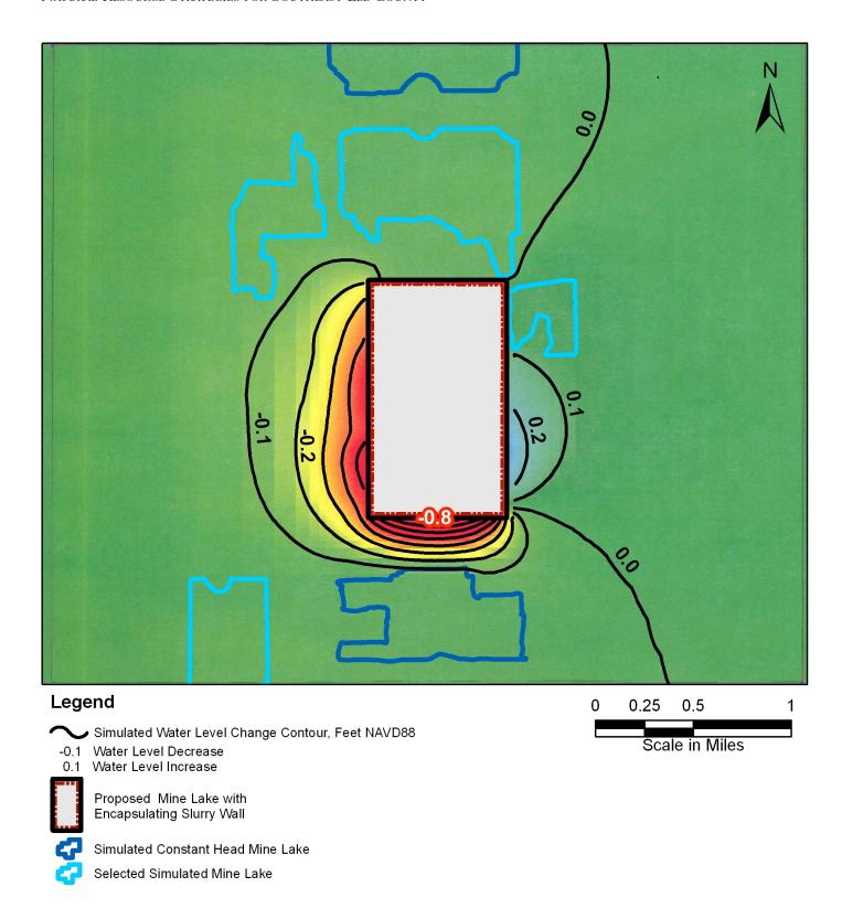
Figure 4.14: Simulated Contours of Water Level Changes for Scenario 5 4.22
