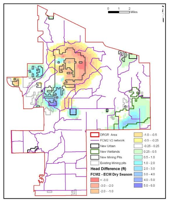
Figure 74. Difference in dry season water table in FCM2 in relation to the LS ECM (Positive values indicate increase in water table elevation in the FCM2).
