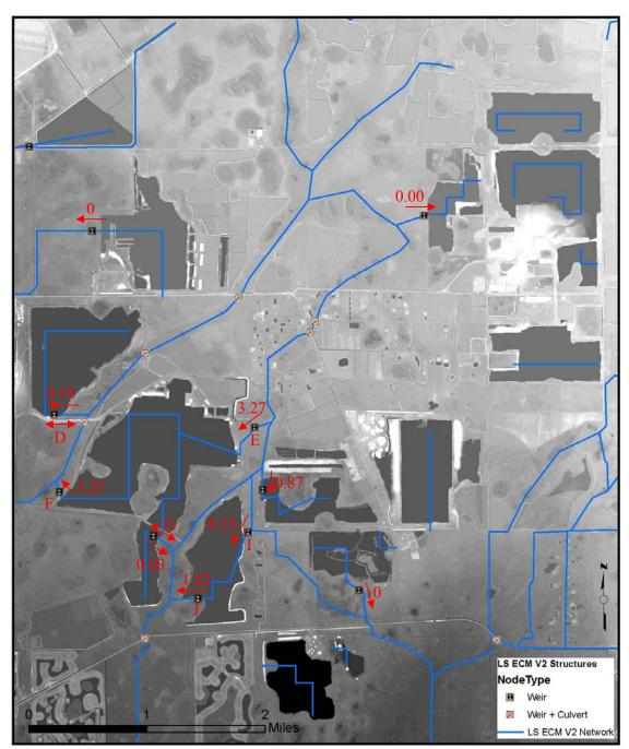
Figure 41. Annual averaged flow rates (in ft<sup>3</sup>/s) in the drainage system around mining pits as obtained from the LS ECM.
