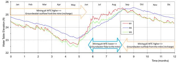
Figure 70. Seasonal averaged water table elevation at locations M1, M2 and M3 in FCM1.
