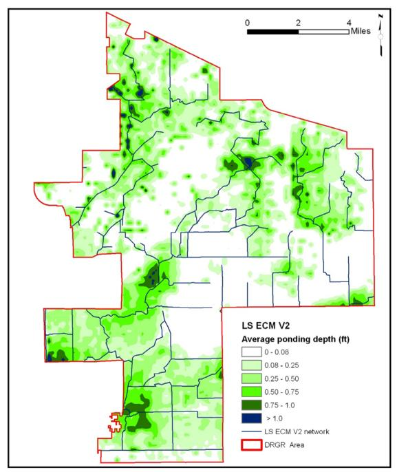
Figure 37. Hydroperiod water depth map obtained from LS ECM.
