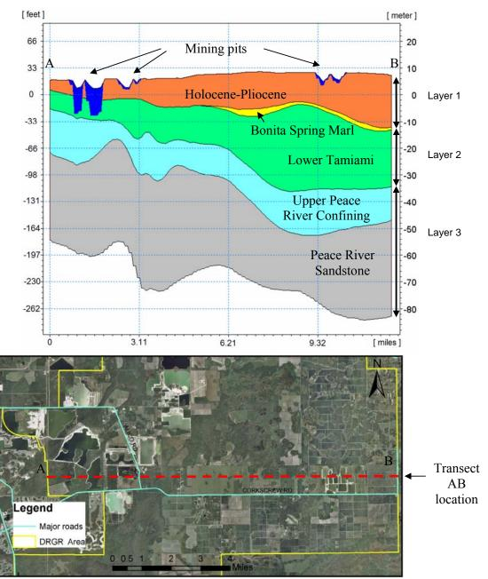
**Figure 12.** Geologic Model and Computational Layers along a transect in the DR/GR Area. <u>Note:</u> blue color in above profile corresponds to the extent of the mining pit conceptual lenses and does not include the water above it, which is conceptualized in the overland component of the model.
