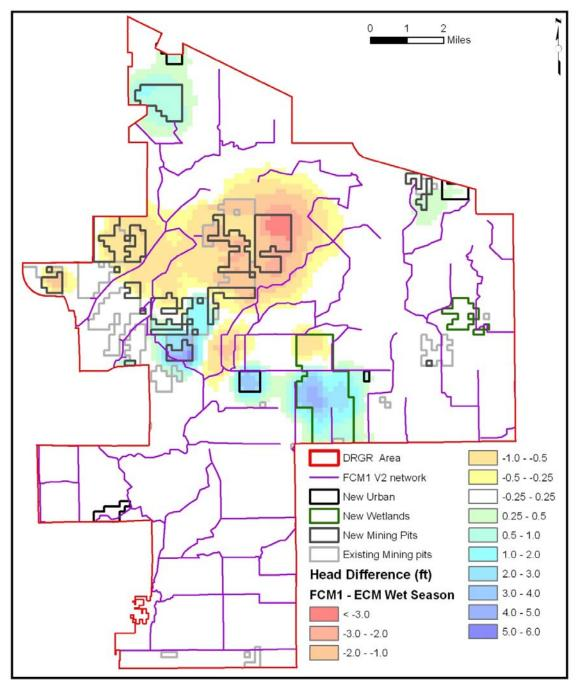
Figure 72. Difference in dry season water table in FCM1 in relation to the LS ECM (Positive values indicate increase in water table elevation in the FCM1).
