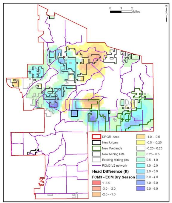
Figure 76. Difference in dry season water table in FCM3 in relation to the LS ECM (Positive values indicate increase in water table elevation in the FCM3).
