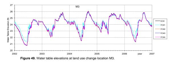
Note: Locations M1 and M3 are close to a new mining pit included in FCM1 and location M2 is inside it. The model predicts that this mining pit recharges the groundwater such that the water table elevation (WTE) in neighboring areas increases during dry periods compared to the ECM. WTE oscillation in location M2 shows a reduction in the seasonal amplitude when located in a mining pit. The corresponding seasonal averaged plots are shown in Figure 70.
