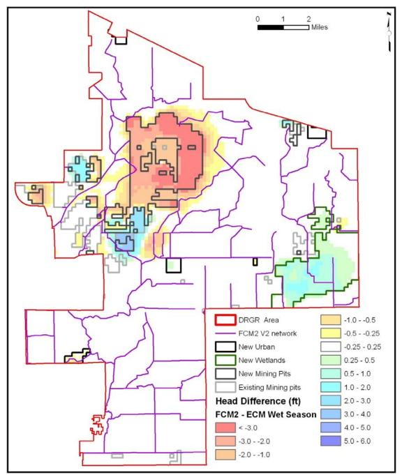
Figure 75. Difference in wet season water table in FCM2 in relation to the LS ECM (Positive values indicate increase in water table elevation in the FCM2).
