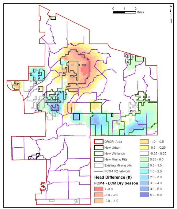
Figure 78. Difference in dry season water table in FCM4 in relation to the LS ECM (Positive values indicate increase in water table elevation in the FCM4).
