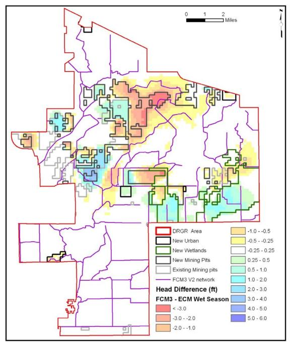
Figure 77. Difference in wet season water table in FCM3 in relation to the LS ECM (Positive values indicate increase in water table elevation in the FCM3).
