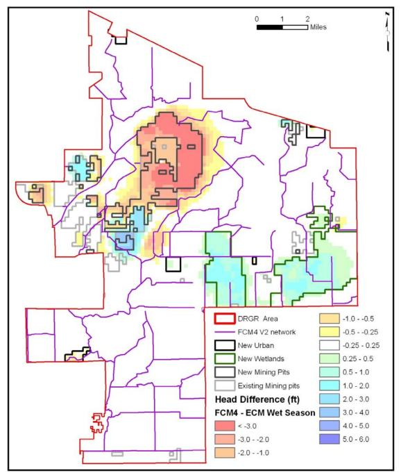
Figure 79. Difference in wet season water table in FCM4 in relation to the LS ECM (Positive values indicate increase in water table elevation in the FCM4).
