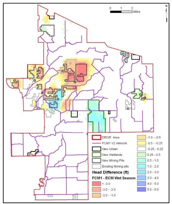
Figure 73. Difference in wet season water table in FCM1 in relation to the LS ECM (Positive values indicate increase in water table elevation in the FCM1).
