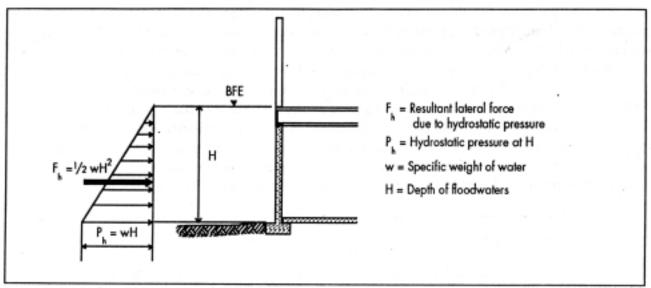
Figure 5. Lateral Hydrostatic Force and Pressure
