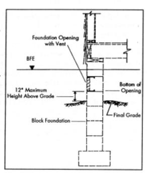
Figure 1. Opening for Solid Foundation Wall
