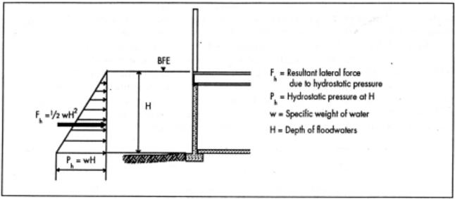
Figure 5. Lateral Hydrostatic Force and Pressure
