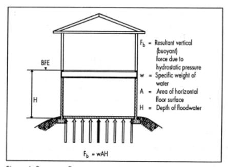
Figure 6. Buoyancy Force
