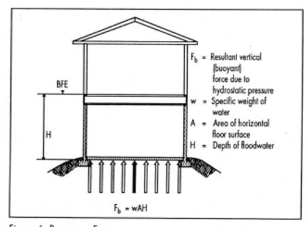
Figure 6. Buoyancy Force
