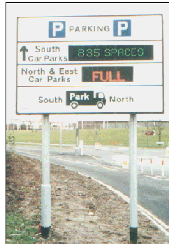
Figure 16, Variable message sign for parking management
