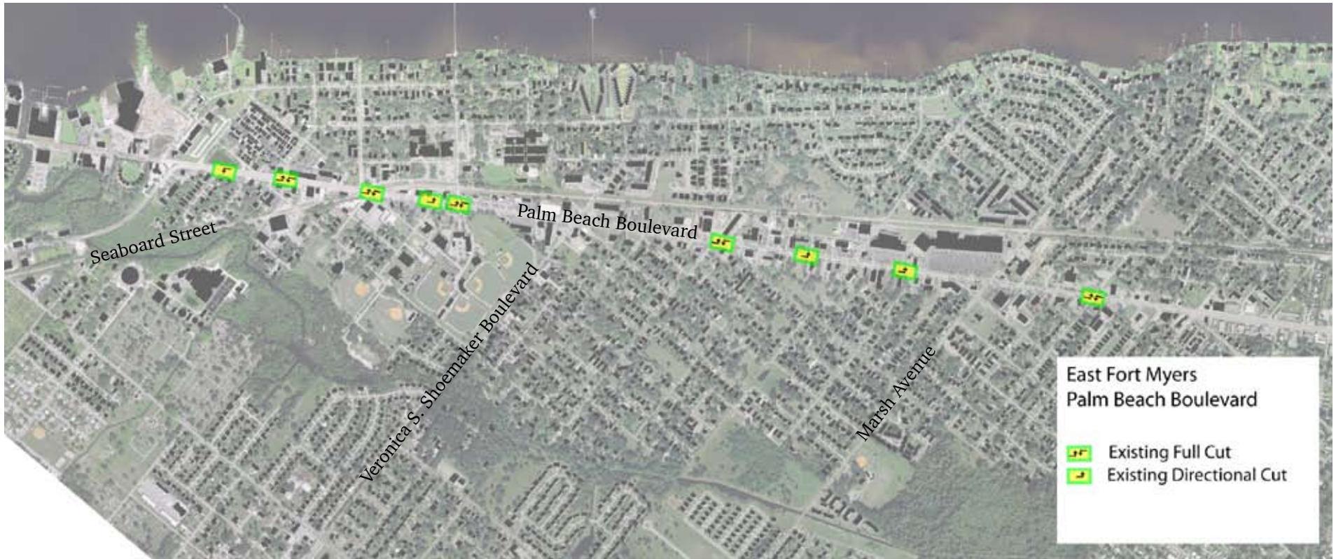
Figure 5.2: Existing Median Openings
