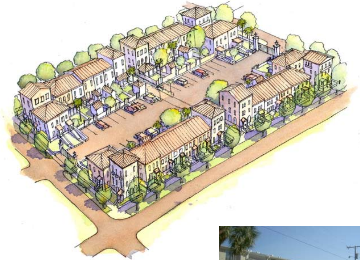
Above: Figure 4.15: A block of townhomes provides parking in the rear so that the streets become pedestrian friendly. Image from the Dr. Martin Luther King Jr. and Veronica S. Shoemaker Boulevards Revitalization Plan .
