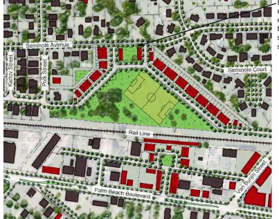
Figure 4.25: The site plan for the proposed Seminole Avenue Park showing adjacent T.O.D. (Transit Oriented Development) and reconnected street network.
