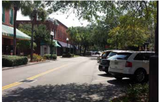
On-street parking creates side friction. Location: Centre Street, Fernandina Beach, FL Source: FDOT
