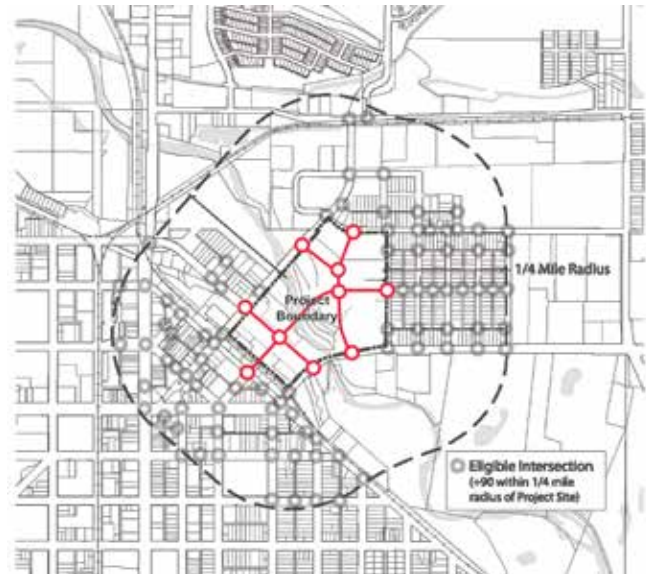
FIGURE A-2 EXAMPLE OF LOCAL NETWORK CONNECTIVITY
