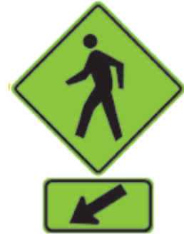
Pedestrian warning sign (MUTCD W11-2) with diagonal downward pointing arrow
