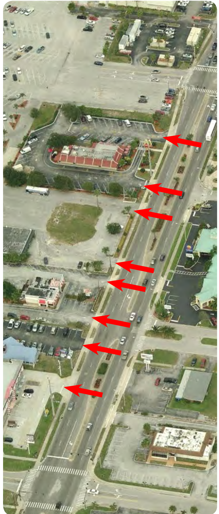
Note all the places a pedestrian could encounter cars entering and existing as they walk along the sidewalk.
