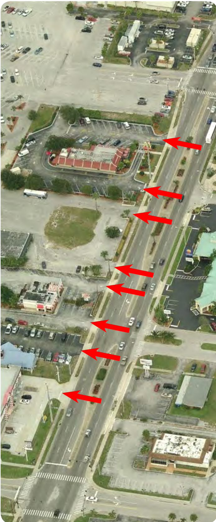
Many of these enter/exit areas could be consolidated.
